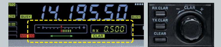
Clarifier Dial and Keys
