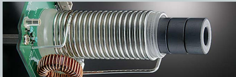
Large-Area (1 1/8" 28 mm) Coil (Actual Size)
